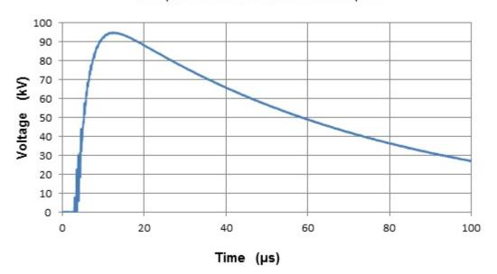
Fig 2.2: Negative lightning impulses captured during lightning impulse testing
